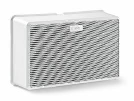
This A/B Cabinet loudspeaker has two independent 6 W loudspeaker systems and is suitable for sound systems where redundancy is requested. In normal situations, both loudspeakers are powered with the same audio signal from independent amplifiers. In case the A-line fails, the other connected loudspeaker receives the signal from line B and the other way around.
